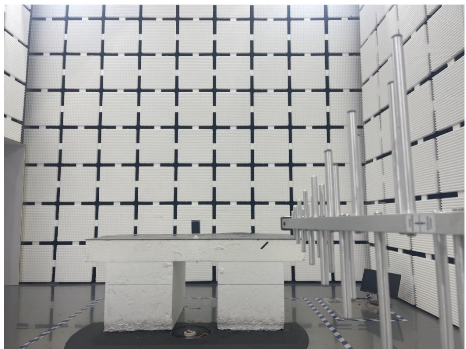
Radiation Emission Test Setup (30MHz to 1GHz) (TM1)
