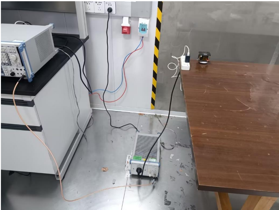
Conducted Emission Test Setup
