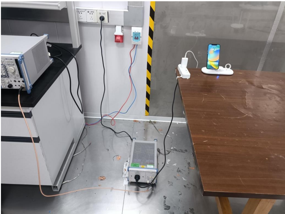
Conducted Emission Test Setup
