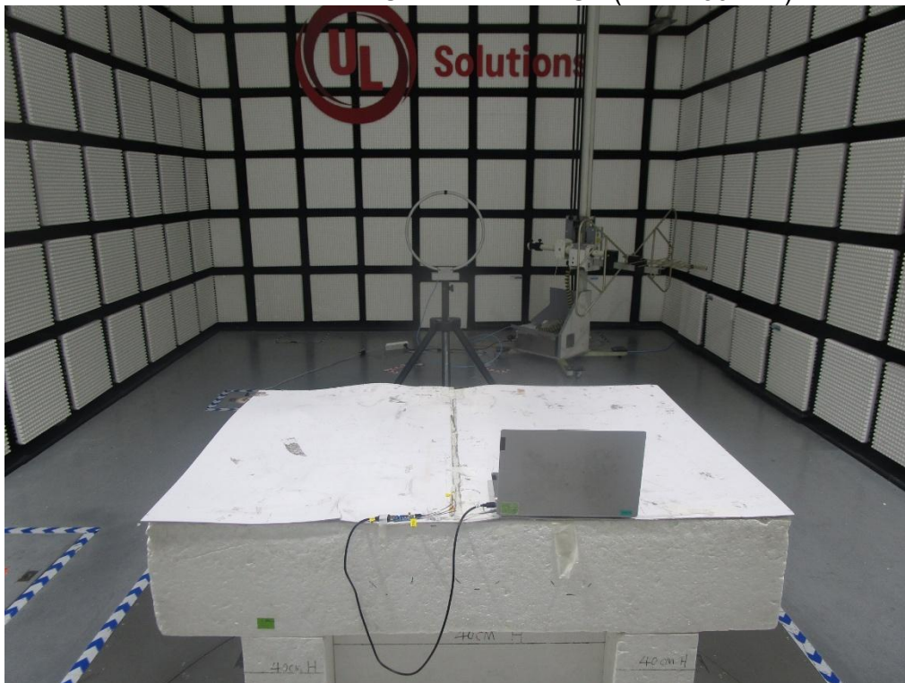
RADIATED RF MEASUREMENT SETUP (Below 30MHz)
