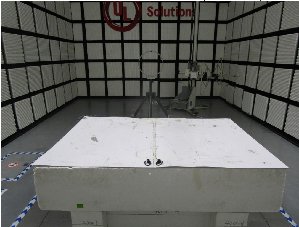
RADIATED RF MEASUREMENT SETUP (Below 30MHz)
