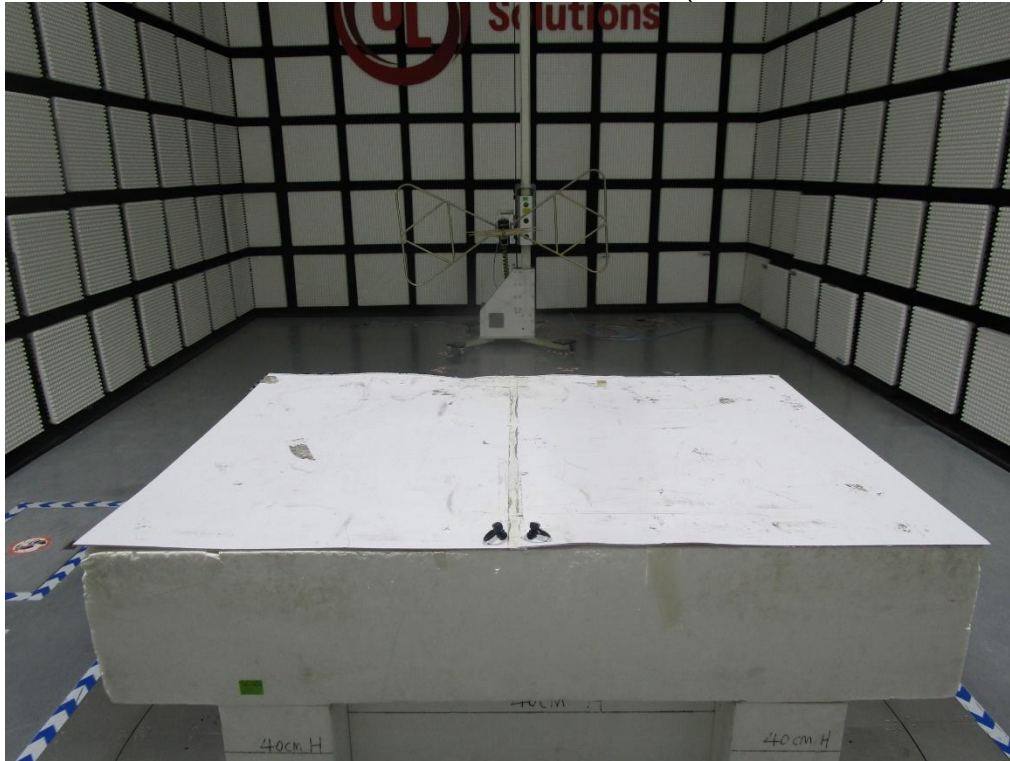
RADIATED RF MEASUREMENT SETUP (Below 30MHz)
