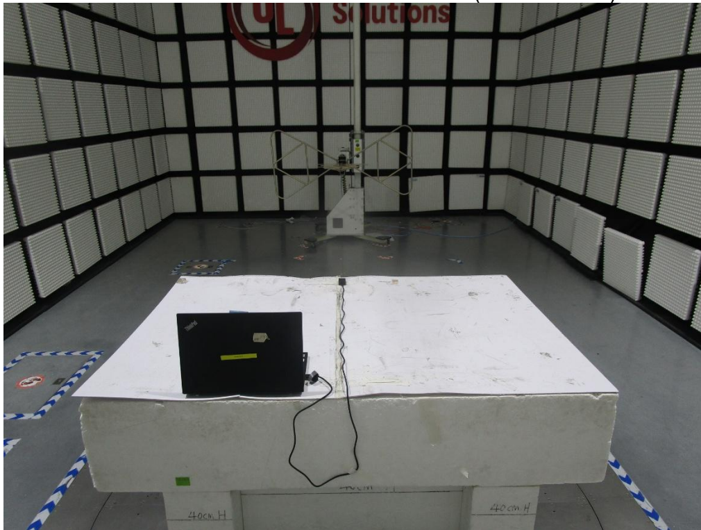
RADIATED RF MEASUREMENT SETUP (Below 30MHz)
