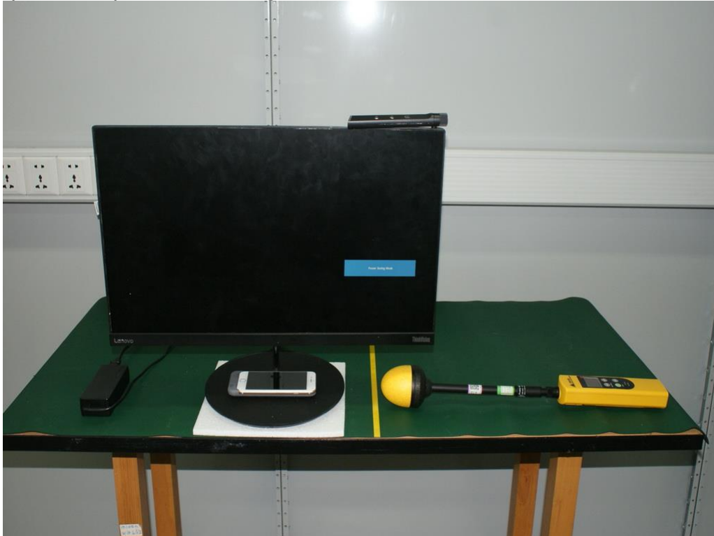
Photograph 1: Setup for Electromagnetic Fields
