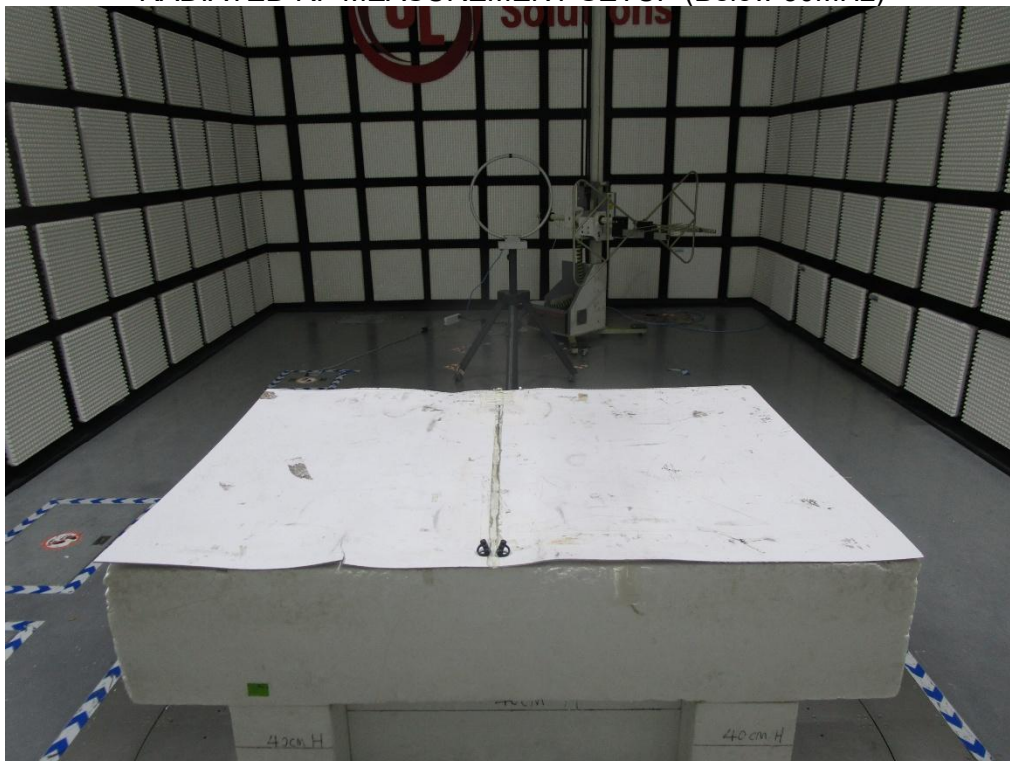
RADIATED RF MEASUREMENT SETUP (Below 30MHz)
