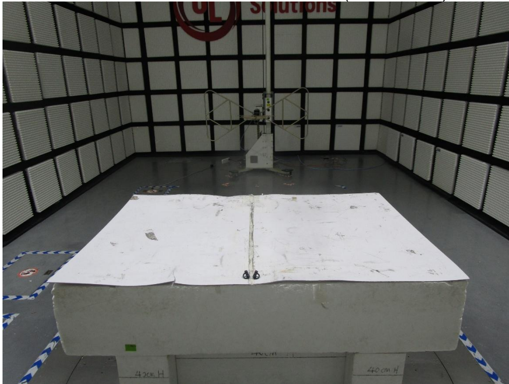
RADIATED RF MEASUREMENT SETUP (Below 30MHz)
