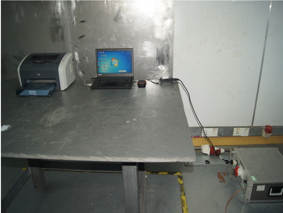
Photograph 6: Set-up for Radiated Emissions, below 1GHz
