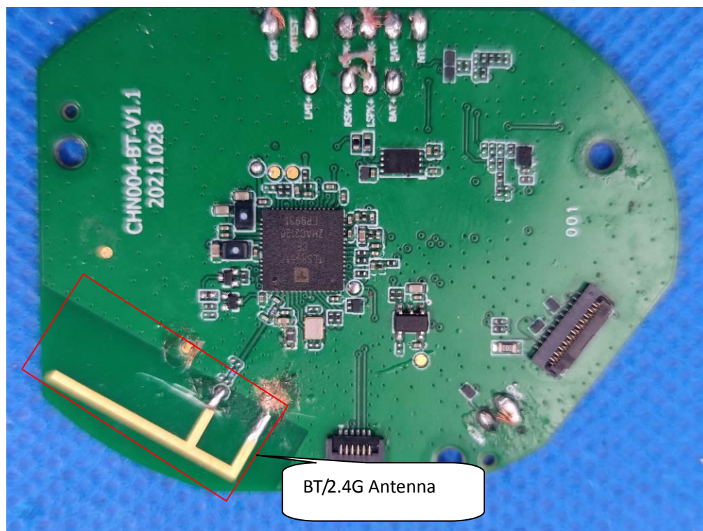
INTERNAL VIEW OF EUT (FIGURE 4)
