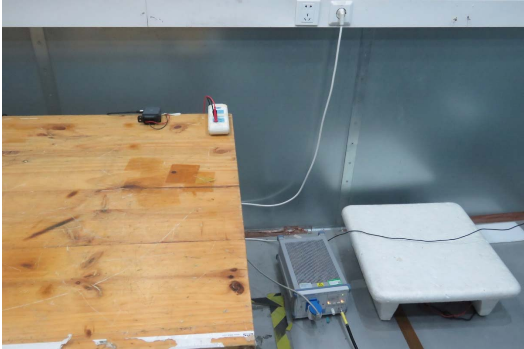
Picture 3 Conducted Emission Test Setup
