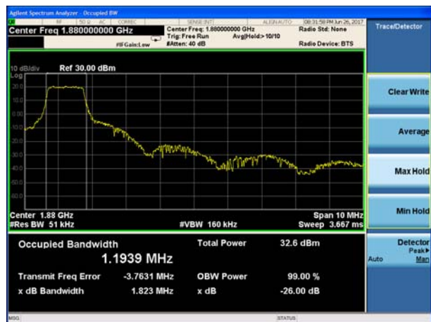
LTE Band 2 15MHz 16QAM CH-Middle
