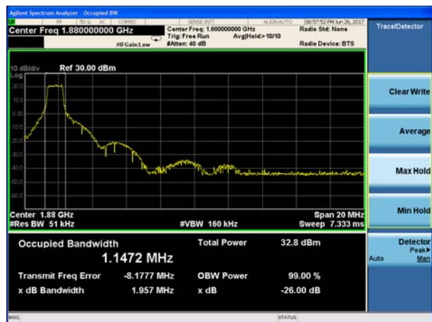
LTE Band 2 20MHz 16QAM CH-Middle
