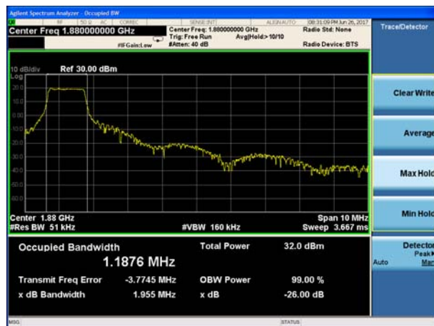
LTE Band 2 15MHz QPSK CH-Middle
