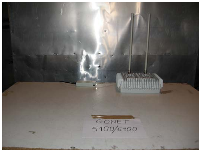
Figure 4. Conducted Emission From AC Power line
