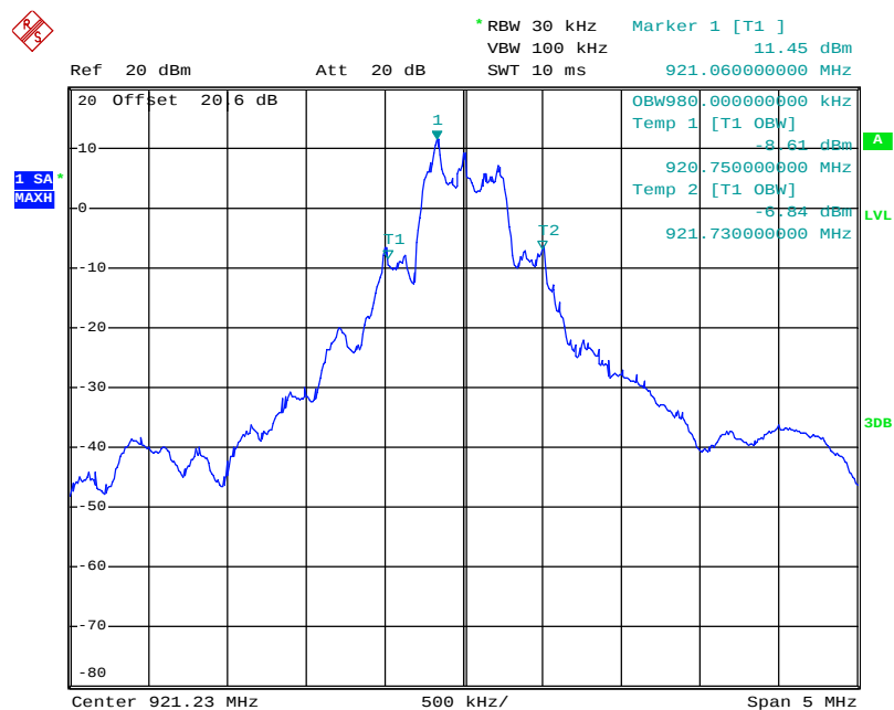
Figure 7.2.2-1: 6dB BW – Low Channel
