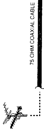
1 COMBINATION VHF/UHF ANTENNA WITH 75 OHM COAXIAL CABLE
