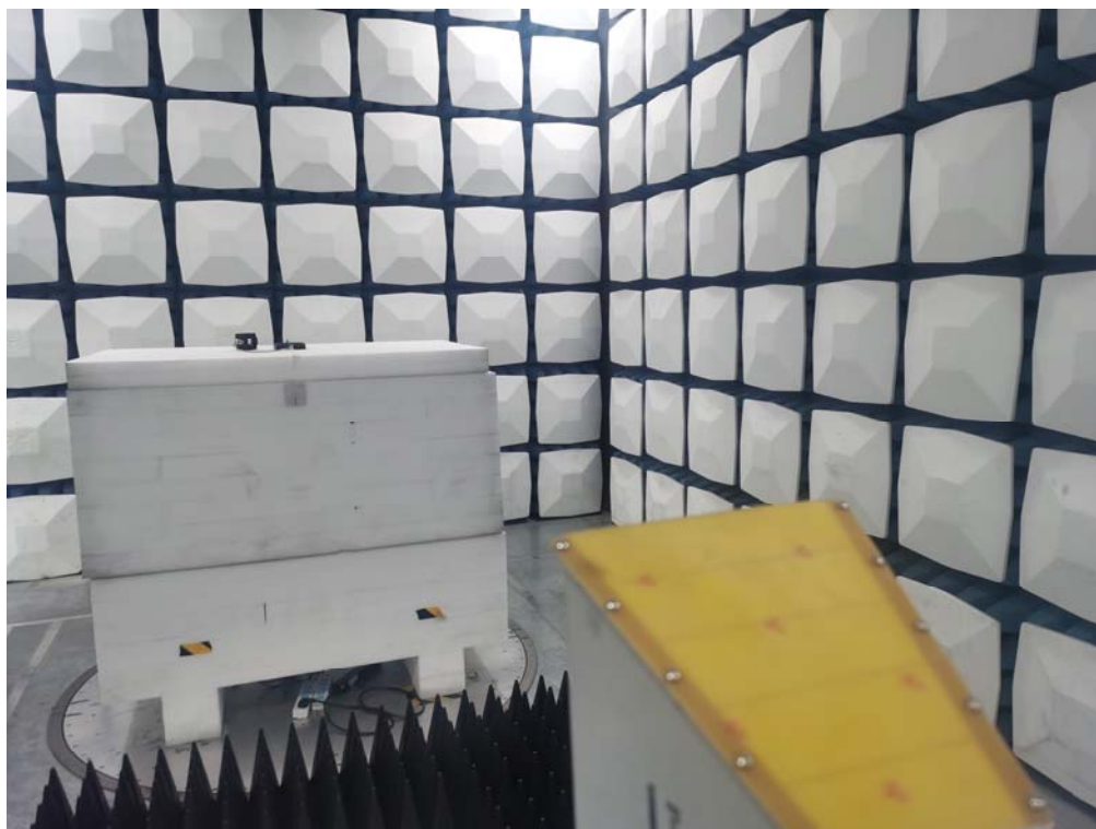
Radiated Emission Above 1GHz View
