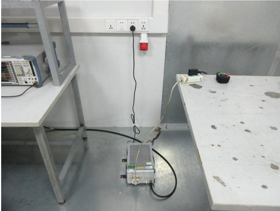
Photo of Conducted Emission Test
