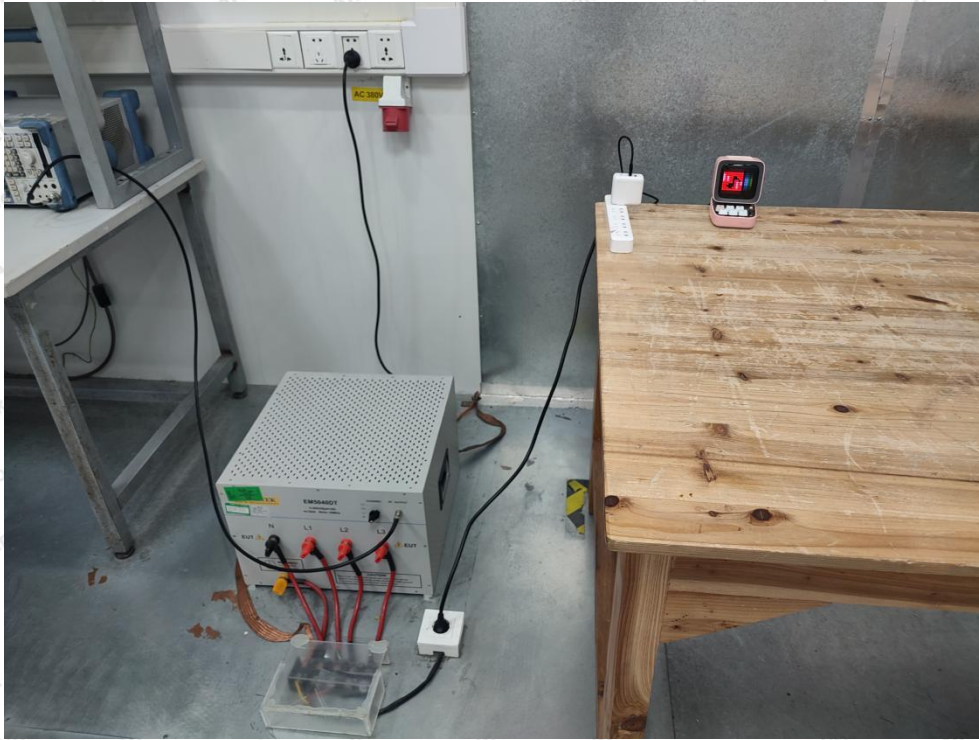
Photo of Conducted Emission Measurement
