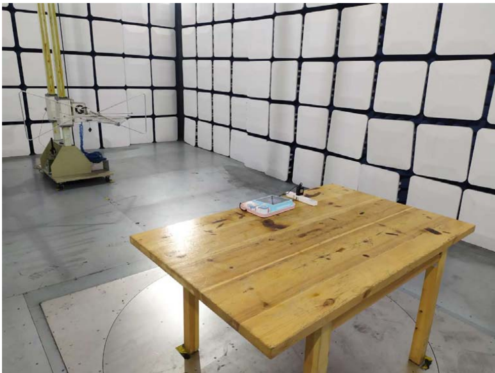
Photo of Radiation Emission Test
