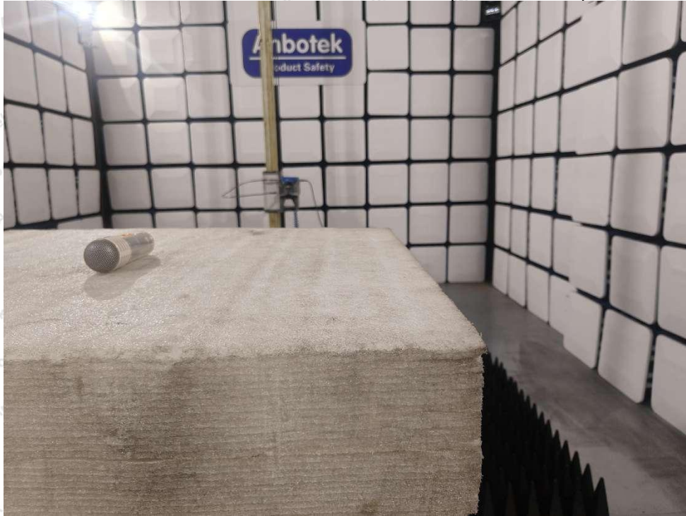
Photo of Radiation Emission Test (above 1GHz)
