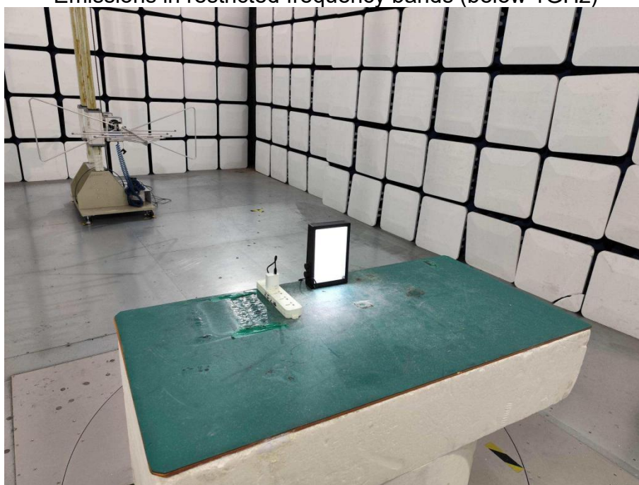
Emissions in restricted frequency bands (below 1GHz)
