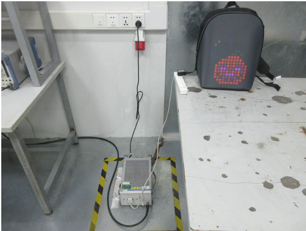
Photo of Radiation Emission Test
