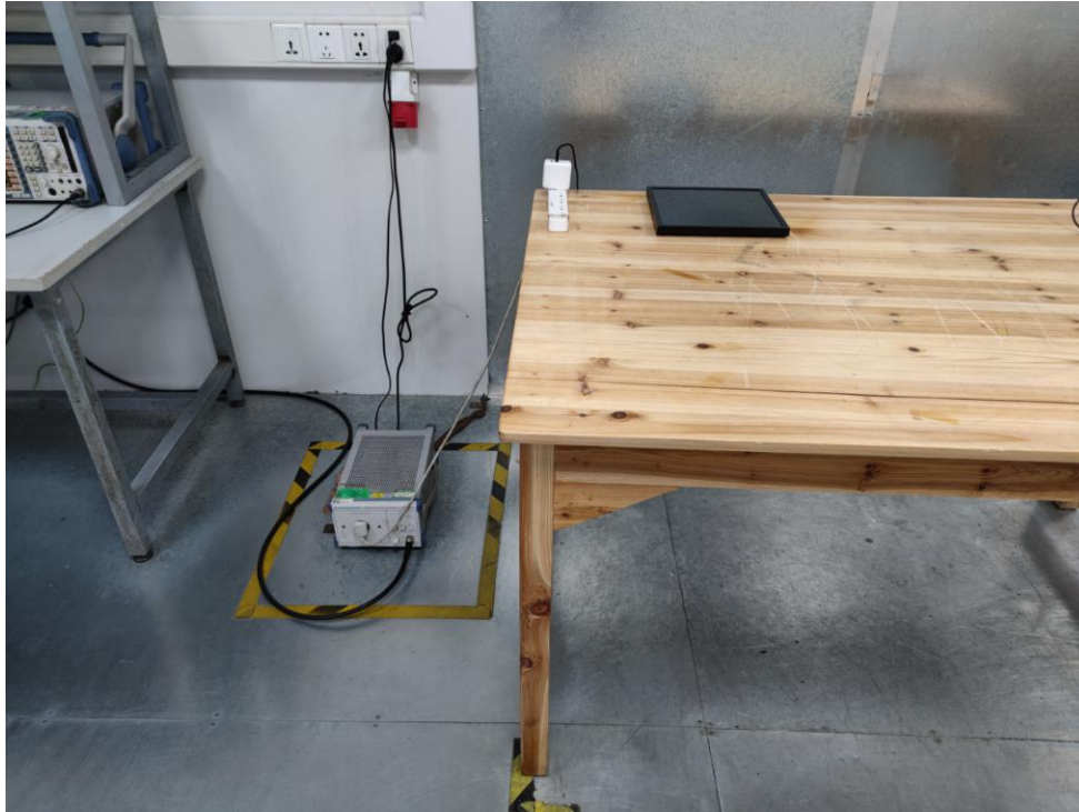
Photo of Power Line Conducted Emission Test
