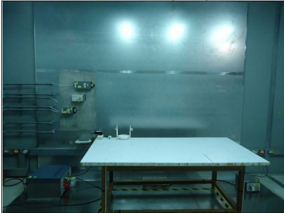
Conducted Emission Test (Mode B2)
