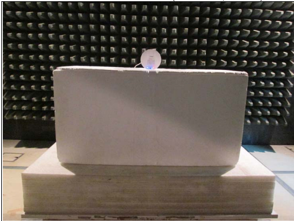
Radiated Emission Test above 1GHz (WLAN 5GHz, Mode B1)
