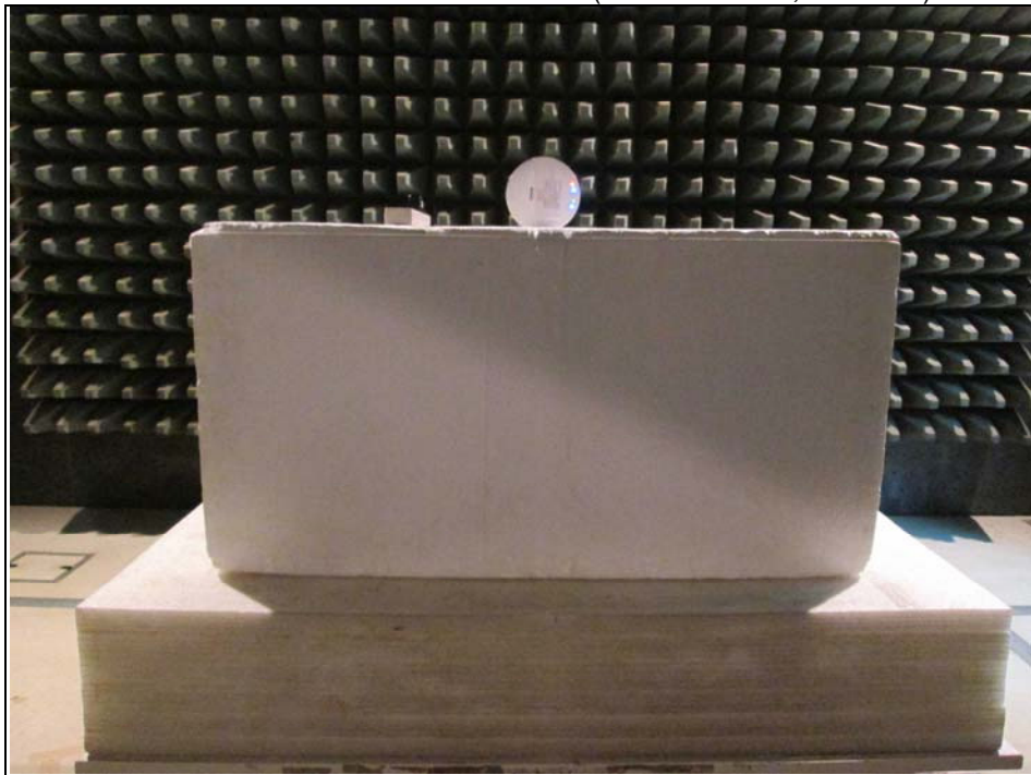
Radiated Emission Test above 1GHz (WLAN 2.4GHz, Mode A1)
