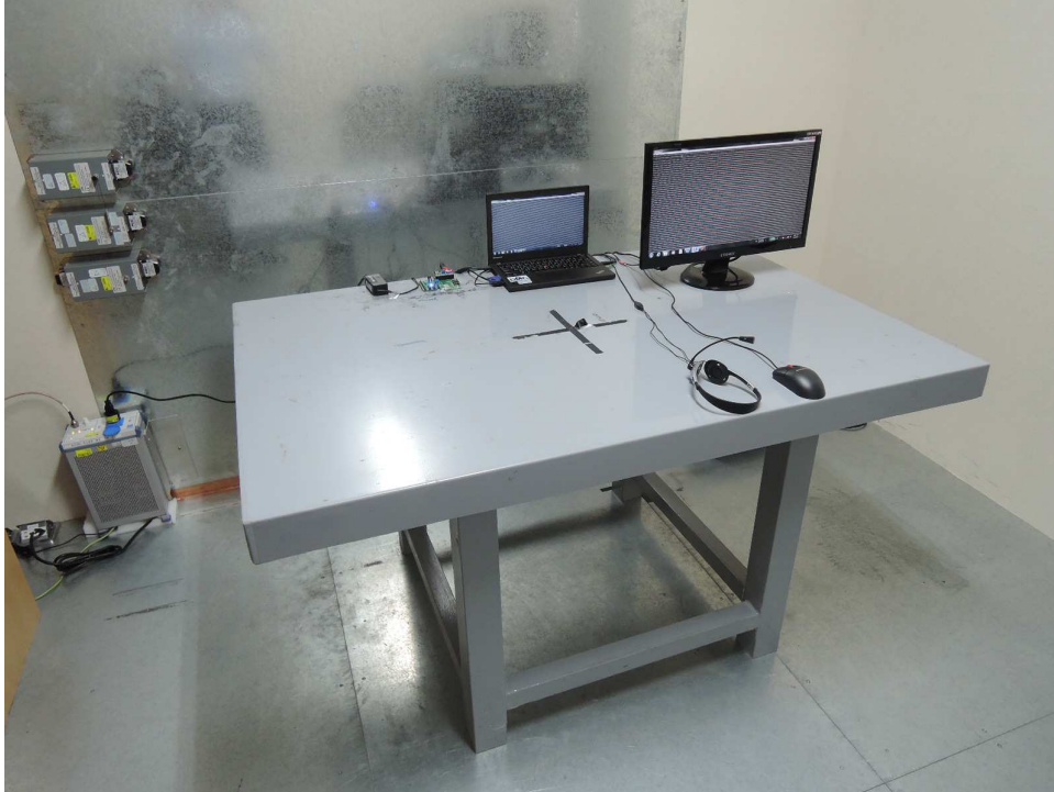
Photograph 8: Set-up for for Mains Conducted testing Front
