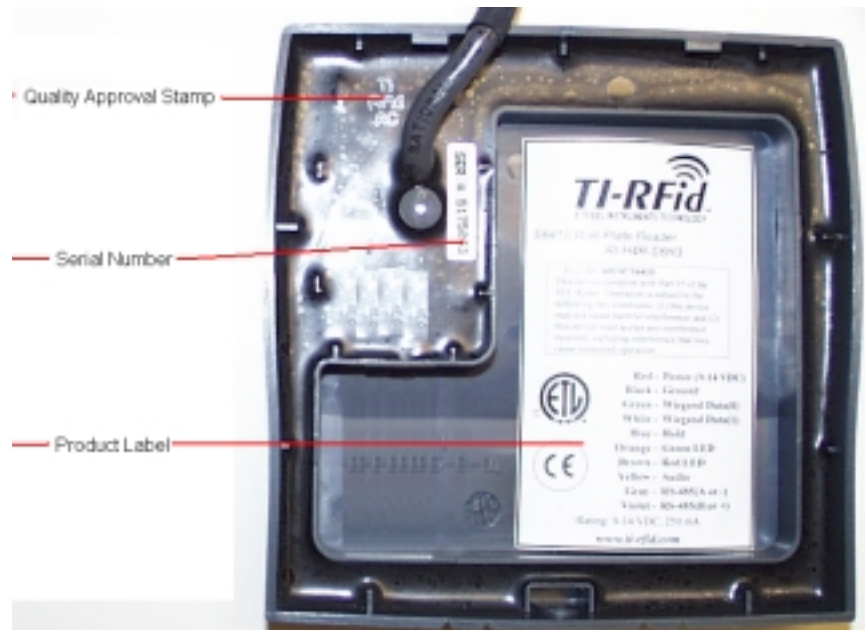
Figure 2. Backside of Wall Plate Readers with back plate removed
