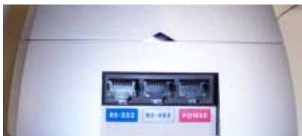
Figure 2: Reader RS232, RS485 and Power Connectors
