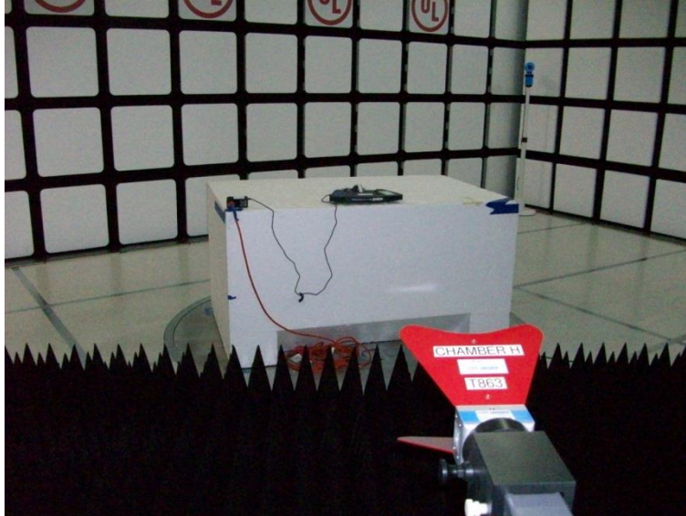
RADIATED FRONT PHOTO (ABOVE 1 GHz)
