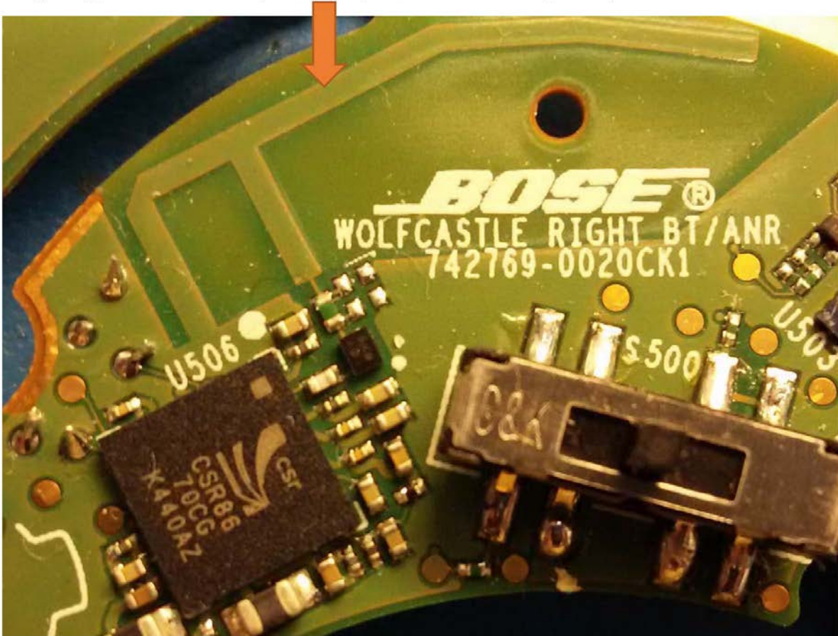
Zoomed in view of Radio PCB, w/ Antenna
