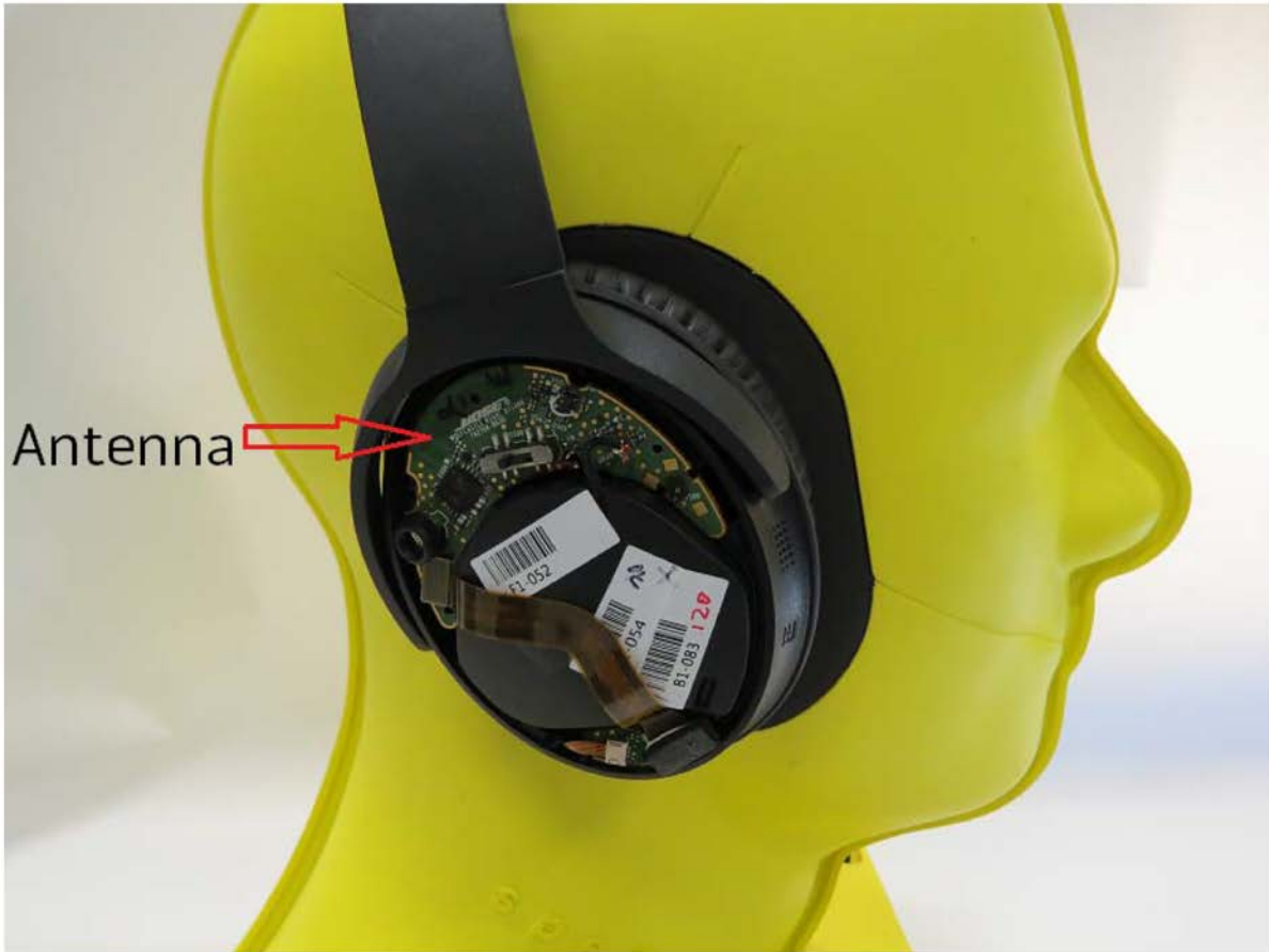
Location of Antenna with Cover Removed
