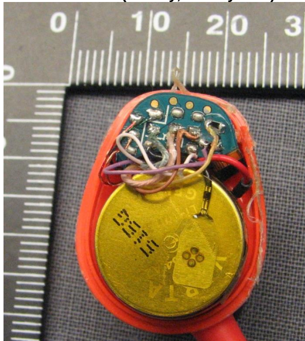
Left earbud (Battery, Battery PCB)
