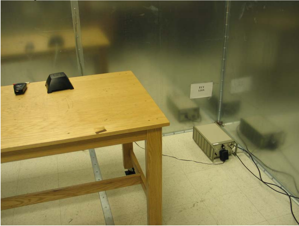
Test setup for conducted emission measurement
