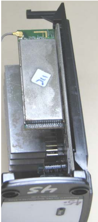
radio control module and partial backside of ML5800 radio module.
