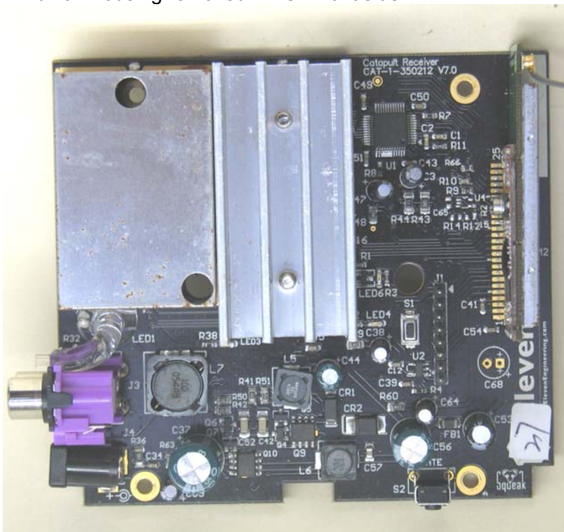
Shield cover for the audio switching amp removed
