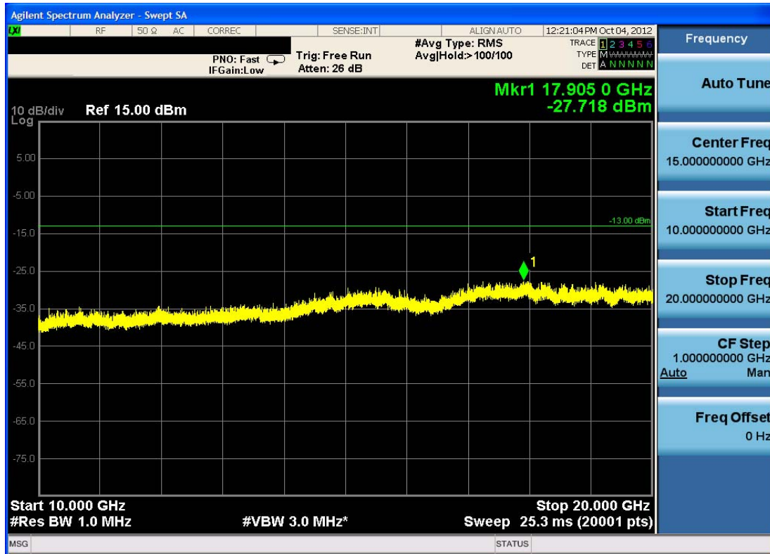
Plot 7-17. Conducted Spurious Plot (PCS GSM Mode – Ch. 661)
