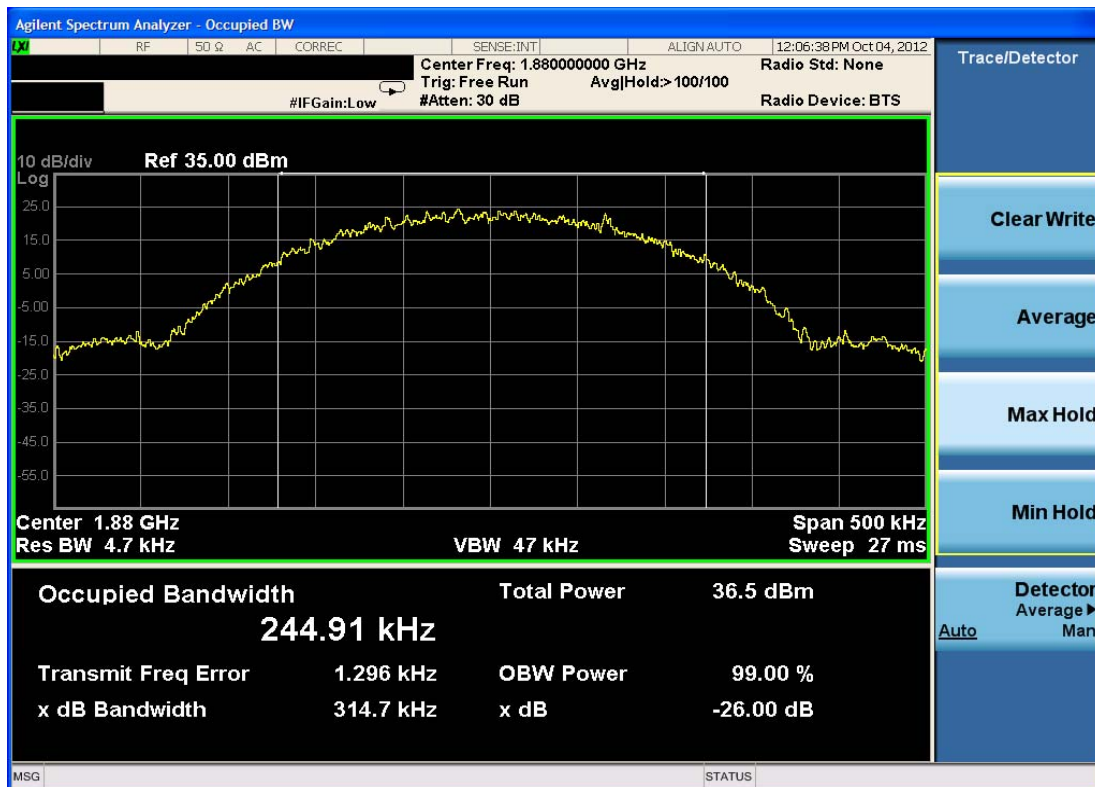
Plot 7-18. Occupied Bandwidth Plot (PCS GSM Mode – Ch. 661)
