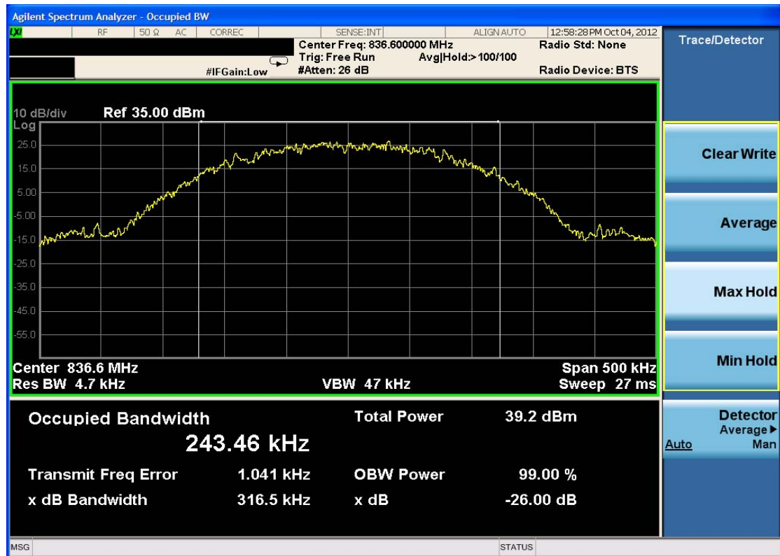
Plot 7-8. Occupied Bandwidth Plot (Cellular GSM Mode – Ch. 190)
