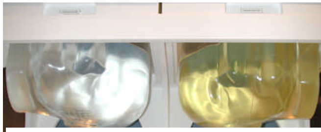
Figure 7.1 Left and Right SAM Phantom shells
