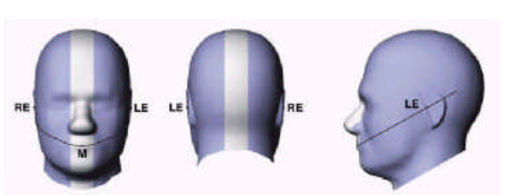
Figure 8.1 Front, back and side view of SAM Twin Phantom
