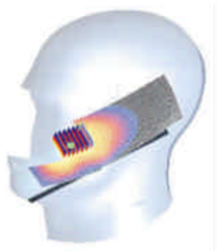
Figure 7.1 Sample SAR Area Scan
