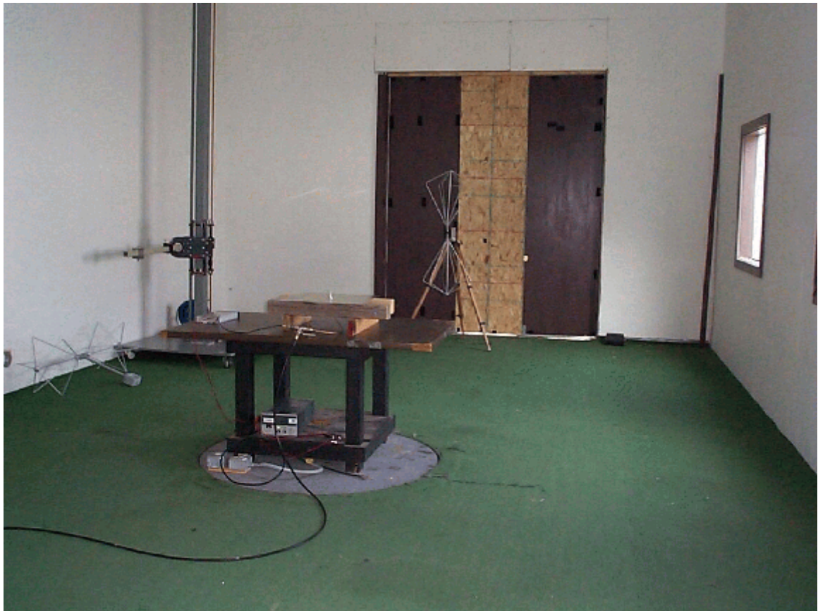
Figure 8-2 Photograph of Field Strength of Spurious Radiation Setup 30 MHz to 200 MHz Vertical Polarization
