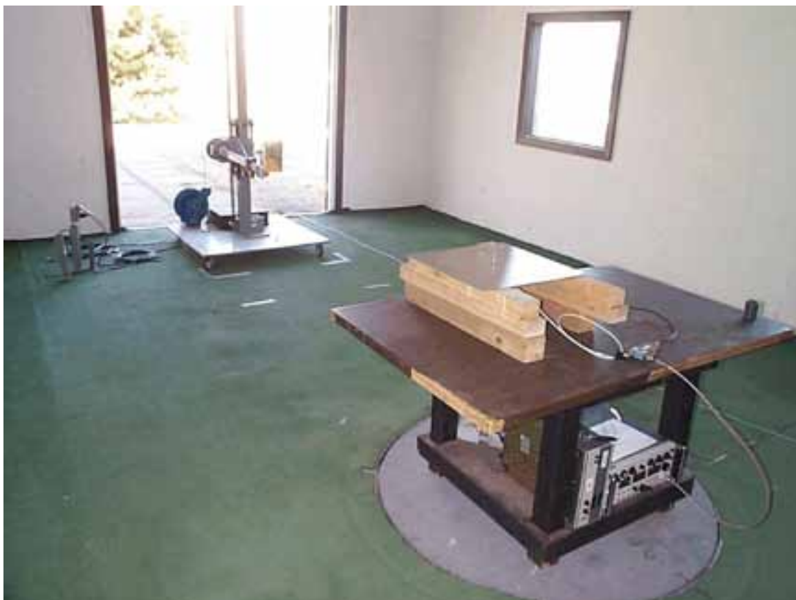
Figure 8-6 Photograph of Field Strength of Spurious Radiation Setup 1 GHz to 11 GHz Horizontal Polarization
