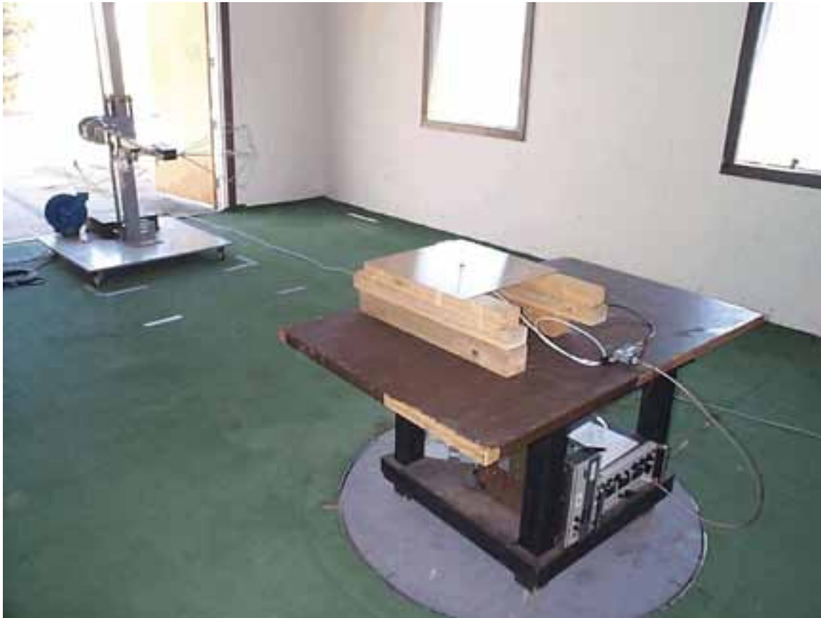
Figure 8-2 Photograph of Field Strength of Spurious Radiation Setup 20 MHz to 200 MHz Horizontal Polarization
