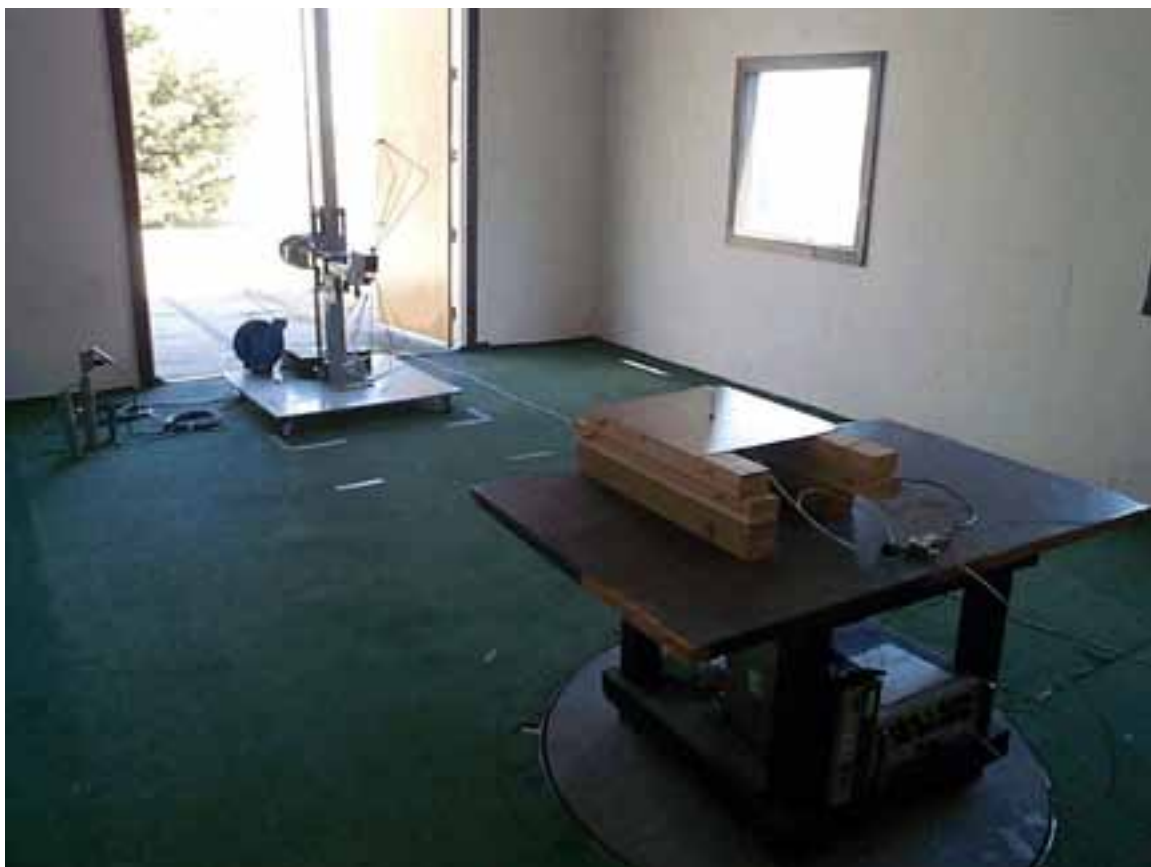
Figure 8-1 Photograph of Field Strength of Spurious Radiation Setup 20 MHz to 200 MHz Vertical Polarization
