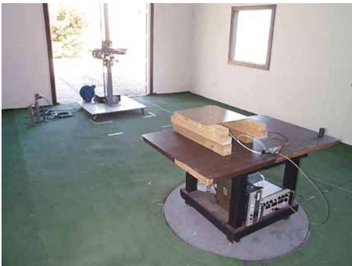
Figure 8-4 Photograph of Field Strength of Spurious Radiation Setup 200 MHz to 1000 MHz Horizontal Polarization
