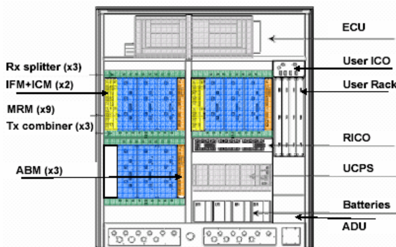
Figure 1- GSM 18000 MCPA BTS Cabinet fully equipped overview ( Open doors )
