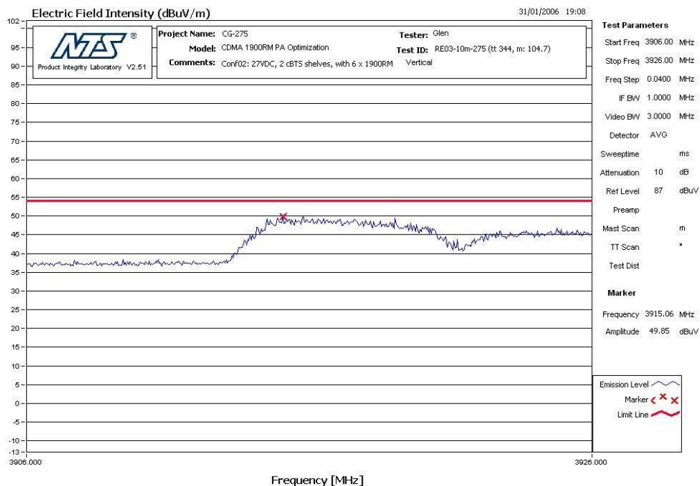
Vertical Compliance Scan @ 3915.06 MHz
