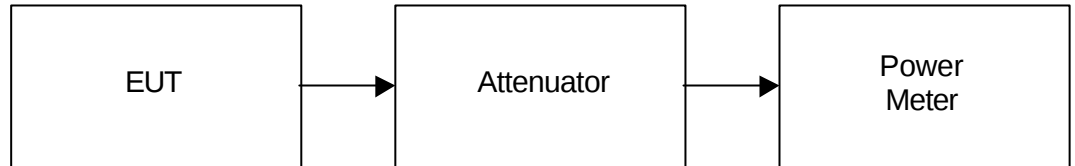
Figure 1 - Measurement Setup for RF Output Power
