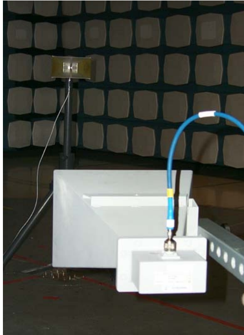
Picture 9: Signal Substitution measurement setup at 3M
