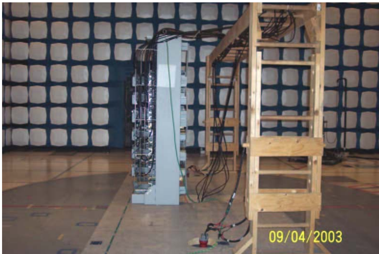
Test setup for the Radiated Emission Right
