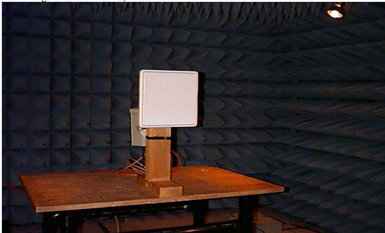
5GHz Large External Antenna, 23.6dBi
