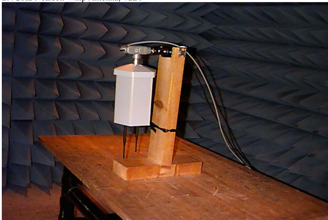
2.4GHz Nearson Whip Antenna, 4dBi
