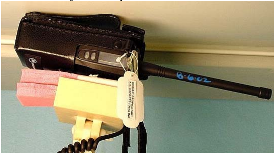
Figure 4. Assessment @ Abdomen; DUT w/ carry case model RLN5383A, NTN5243A, NAD6502A, and HMN9030A against the flat phantom
