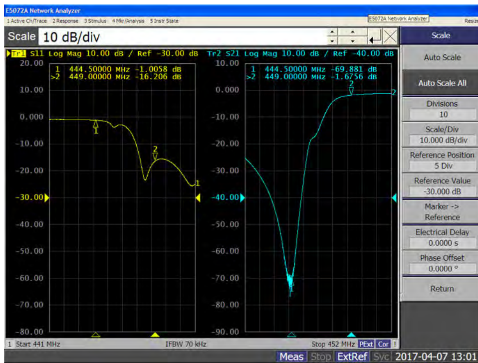
Figure 25: Example for HIGH Port Tuning of the UHF Duplexer
