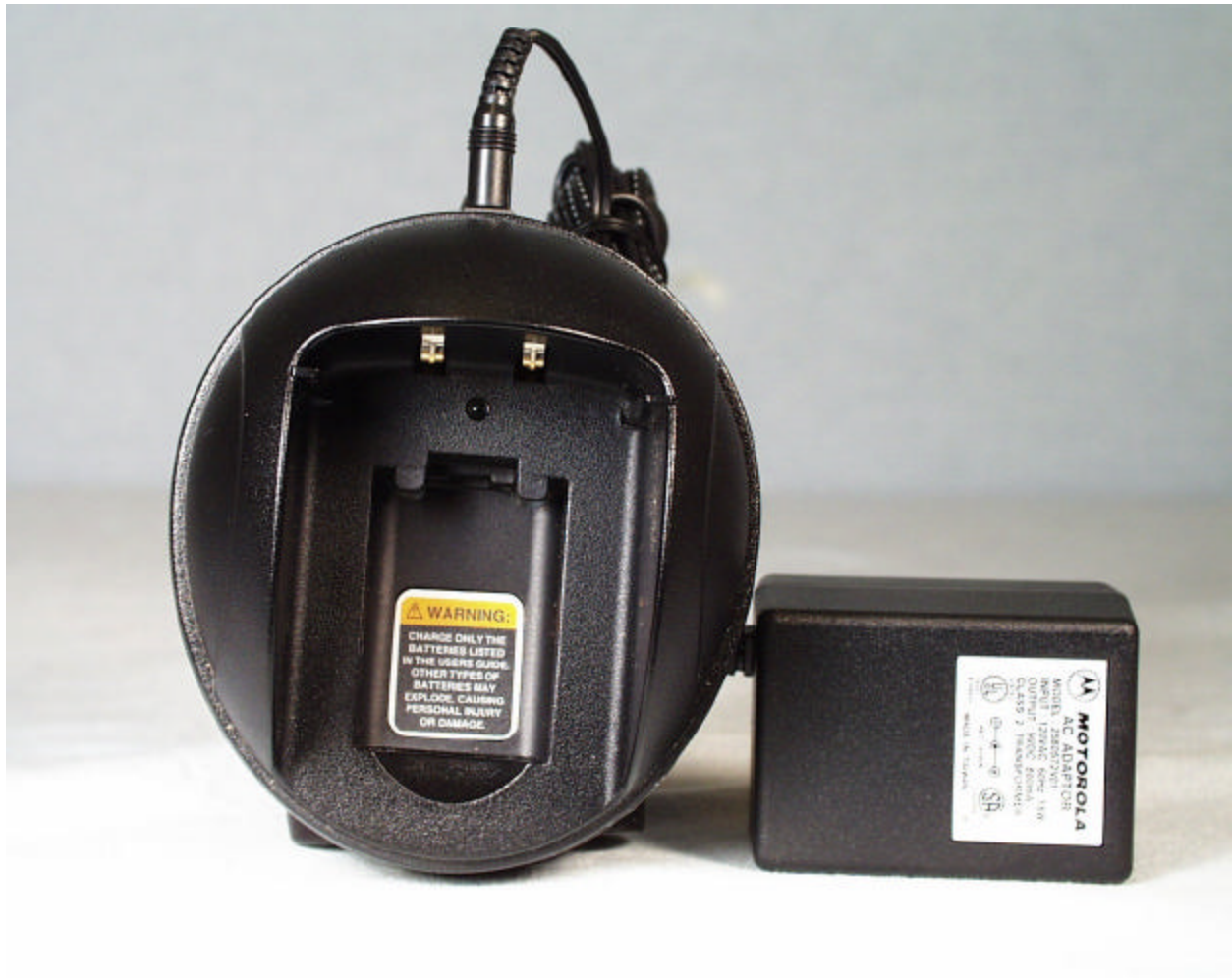
Front View of the Single Charger
