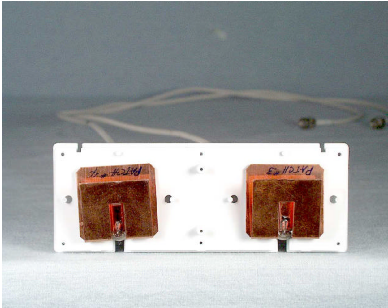
Inside of External Antenna Unit
