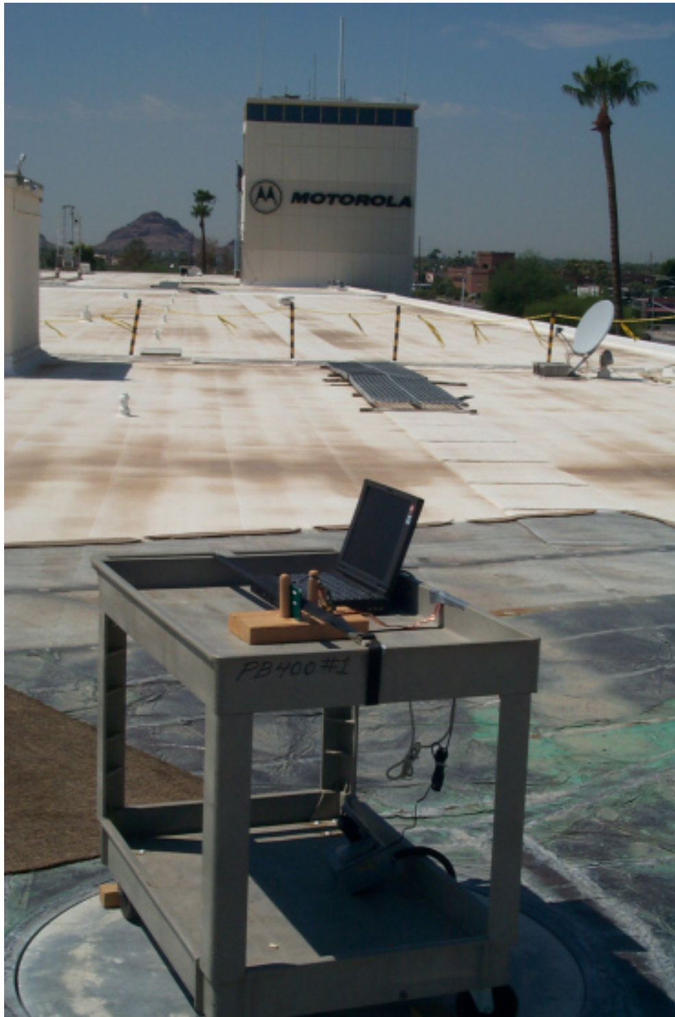
Figure E – 4 Radiated Spurious Emissions Test Setup, OATS
